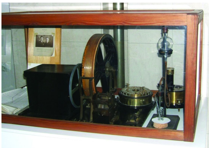
Figure 8. One of the First Polarographs Equipped with a Dropping-Mercury-Electrodes Heyrovský Used. Photograph by Roger Rea.
