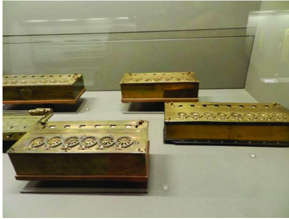
Figure 14. Examples of Blaise Pascal's 1642 calculating machine. Its principal innovation seems very basic to modern eyes: it adds or subtracts, carrying over automatically. Photograph by Mary Virginia Orna.
