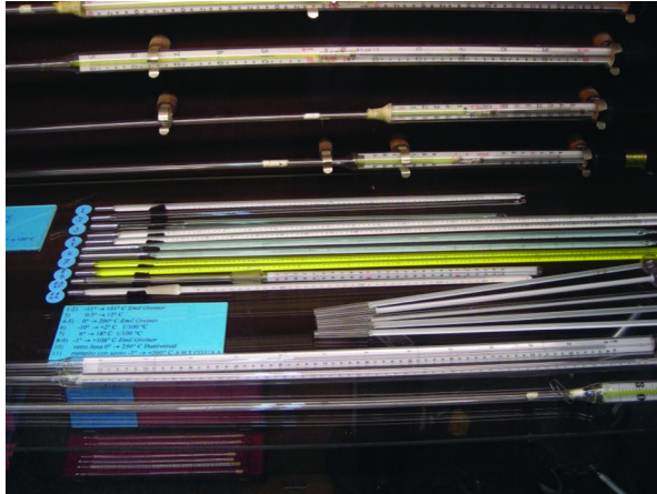
Figure 2. Precision thermometers dated 1882-1887 from the firm of Goulaz of Paris, some measuring to a hundredth of a degree C. Photograph by Mary Virginia Orna.
