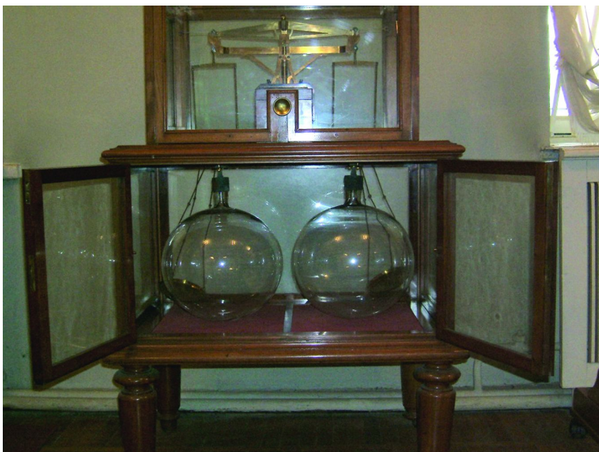
Figure 20. Double-Pan, Equal-Arm Balance Mendeleev Used in Studying the Composition of Gases. Photograph by Roger Rea.
