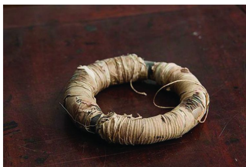
Figure 4. Faraday's Electromagnetic Induction Ring, First Used on 29 August 1831.
