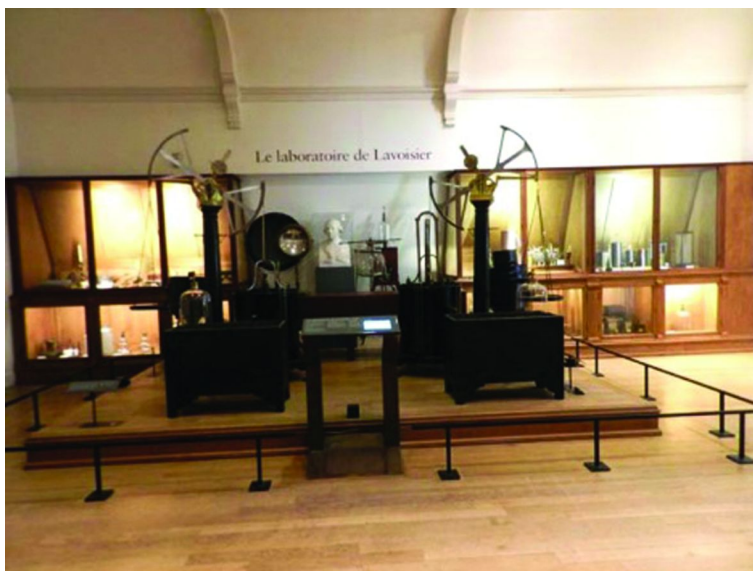
Figure 13. A simulated laboratory of A. L. Lavoisier; note the two gasometers for weighing gases using the precision balances built for that purpose. Photograph by Mary Virginia Orna.
